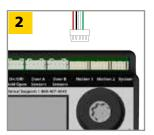
Plug Eagle Harness(es) into hub port labled **Motion 1** and, if applicable, **Motion 2**.
