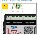
Plug Door Control Harness into hub port labeled **Door Control A.**
