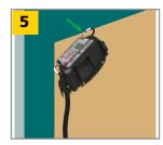
Plug in Slave Sensor Harness at the upper most port on sensor.
