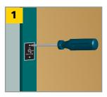
Determine mounting location, apply mounting template, drill holes.
