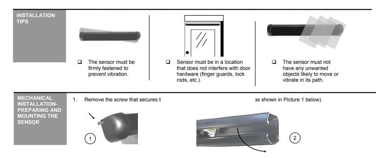
2. Remove the plastic lens by pulling the lens out from the top of the extrusion (as shown in Picture 2 above). Do not use a screwdriver to pry the lens, as cracking may occur.
