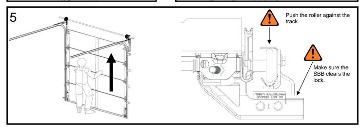
NOTE: The location of the lock is critical. Canimex cannot be held responsible for device misinstallation.
