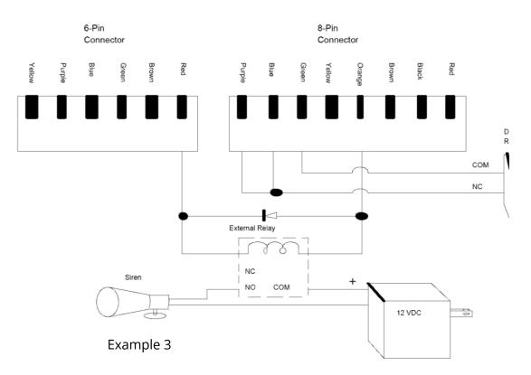
B. Installation of reed switch (normal open), external relay (duress)
