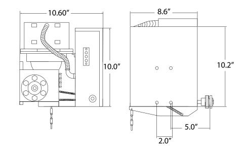
PowerMaster model MGJ Medium Duty Gear reduced jackshaft type operator is rated 1/2 HP, 115 VOLTS, 1 PHASE, for use on Rolling Service Doors, Rolling Grilles, and counter shutters that will be operated up to 10 cycles per hour.
