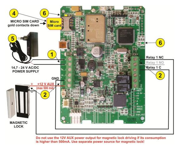
Picture 2: Connection diagram – magnetic lock
