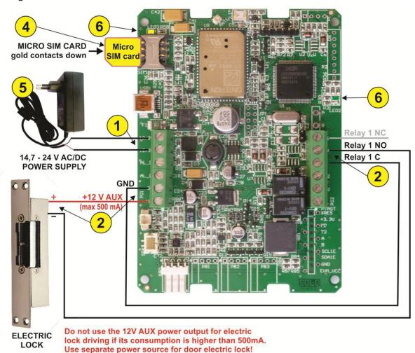
Picture 1: Connection diagram – electric lock
