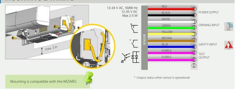
Sensor connectivity (power and relays) must utilize only the supplied harness.
