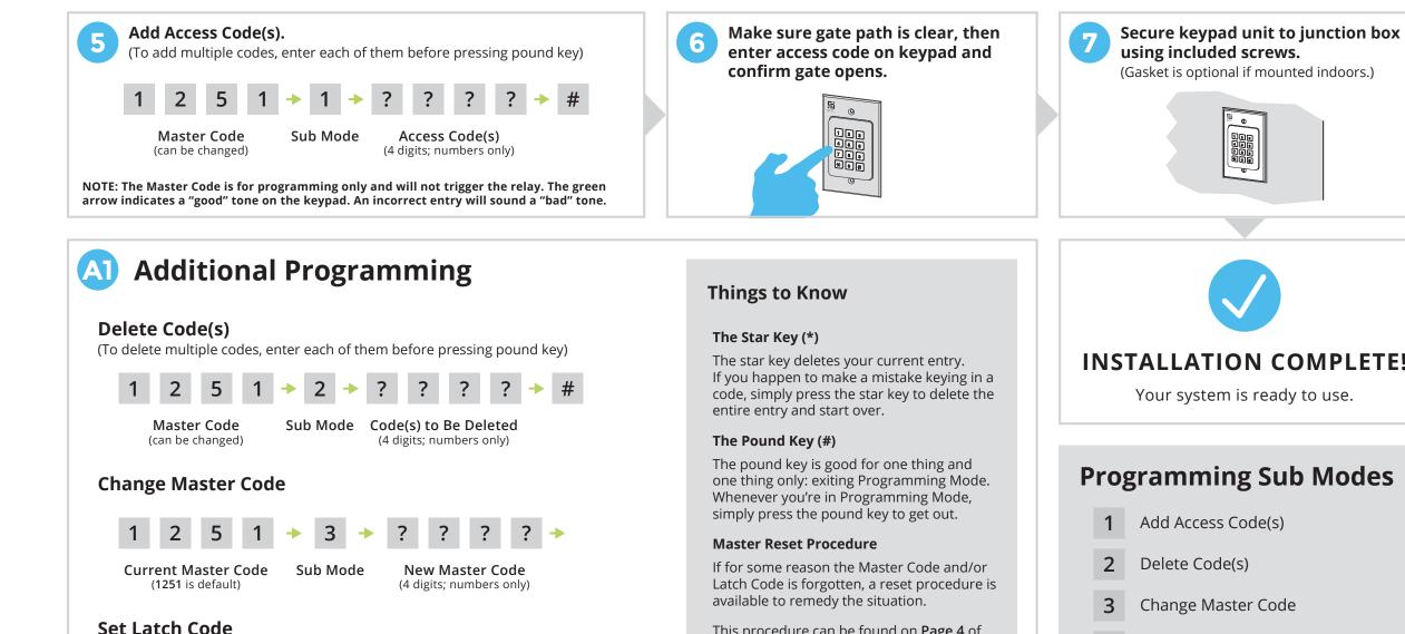
Master Code (can be changed) Sub Mode Latch Code (4 digits; numbers only) This procedure can be found on Page 4 of this guide.
