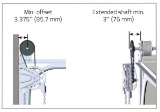
Chain hoist may be mounted on either side of the door
