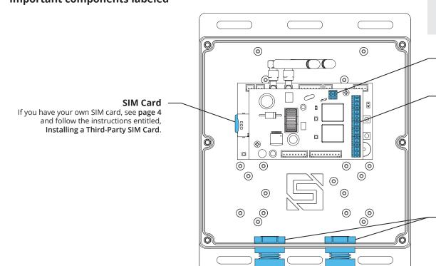
Unit shown with cover removed. Internal wiring not shown for clarity.
