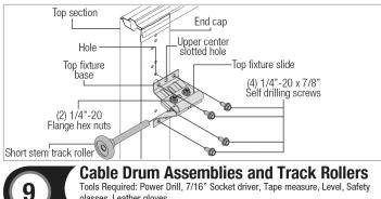
Tools Required: Power Drill, 7/16" Socket driver, Tape measure, Level, Safety glasses, Leather gloves
