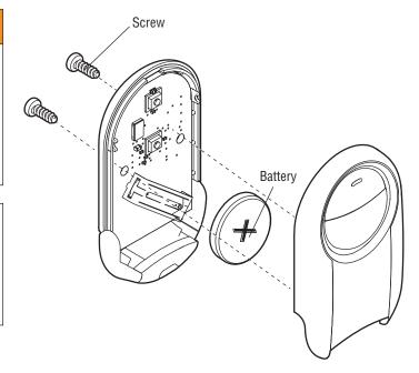
Dispose of batteries properly. Replace ONLY with 3V CR2032 coin batteries.
