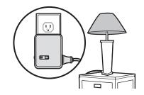
**3** Press and release the LEARN button on the module (the LED on the module will light).
