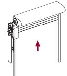
**2** Press and hold bottom button on the remote control until the blue LED stays solid (approximately 15 seconds) then release the button.
