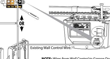
**NOTE:** Wires from Wall Control to Garage Door Opener **ARE** polarity sensitive. Be sure to reattach to the proper terminal should they become detached. Wall control should light when wired correctly.
