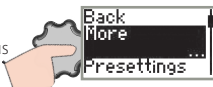
Select More to go to next level: - basic settings - advanced settings - diagnostics
