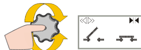
To adjust contrast, push and turn the grey button simultaneously. During normal function only.
