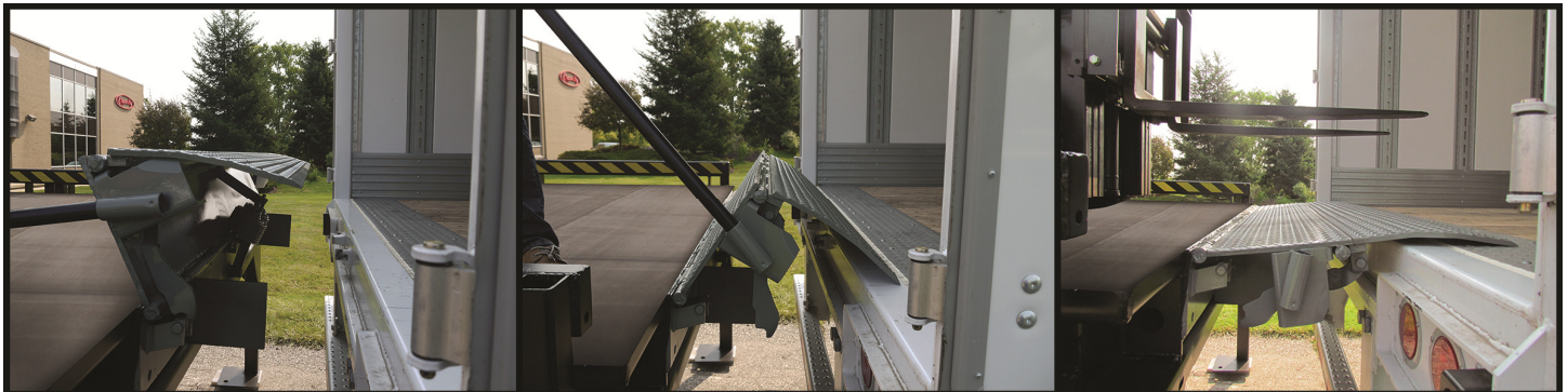
Simply pull back the handle and the lip will mechanically lift over the dock height. Then, a slight forward push of the handle will position the lip onto the truck floor.
