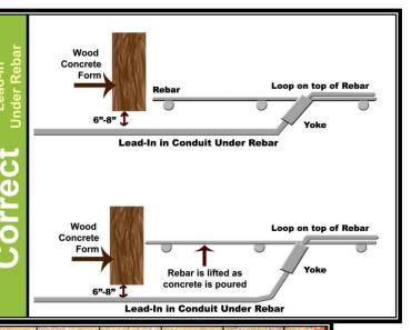
In the picture to the right notice how the "Correct" loop is offset from the rebar pattern. The loop is coming in contact with the rebar as little as possible.
