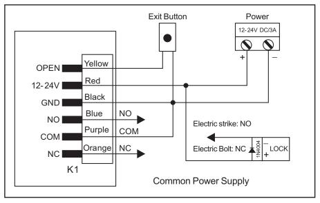
Attention: Install a 1N4004 or equivalent diode is needed when use a common power supply, or the keypad might be damaged. (1N4004 is included in the packing)
