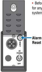
• Before resetting a hard shutdown, determine why the shutdown occurred. Inspect the gate for any obstructions along its path that could have activated the inherent entrapment sensing system. Inspect the gate and gate hardware.
