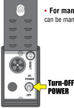
• For manual FAIL-SAFE gate operation, turn power to the operator OFF. Once ALL power is OFF, the gate can be manually operated.
