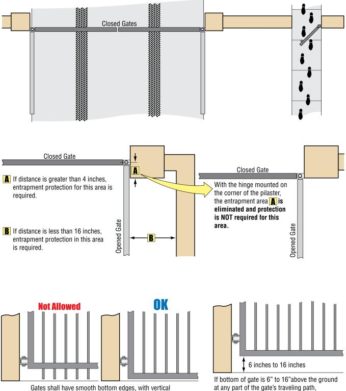
Gates shall have smooth bottom edges, with vertical bottom edged protrusions not exceeding 0.50 inches.
