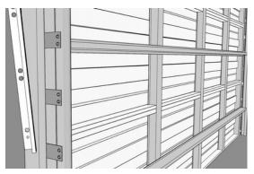
The 90° LED retainer is typically installed on the door track itself. Drill out 3 large holes in the LED retainer's flange (just over the diameter of your existing screws) where the door track screws or nuts are located. Connect the retainer to the door guide tracks using the 3 existing screws.
