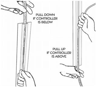
If the LED Controller is installed above the retainers, insert the wire end of the LED strip into the bottom end of the lower retainer. With one hand guiding it from the bottom, pull the wire straight up along the length of the track. If the LED Controller is installed below the retainers, do the same in the other direction. Once you get far enough, you will need an assistant to continue pulling the LED strip through the track until you have reached the desired length.
