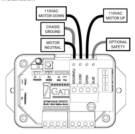
Some door operators do not use circuit boards or provide output relays that can be used to determine fully-open and fully-closed statuses. We connect directly to the motor control leads to determine door movement and direction.
