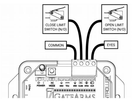
The L3 does not support monitored safety eyes. Thus the default configuration should work as expected.
