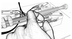
6. Attach the green spaded wire to the "Fully Open" limit switch's available spade terminal.
