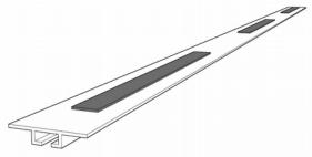
Ensure that all pieces of the retainer are installed straight, preferably by using a level.
