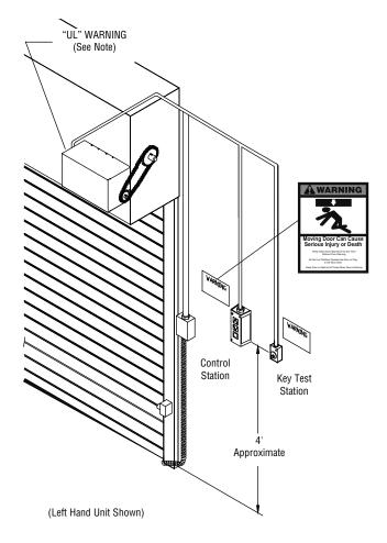
**NOTE:** The "UL" Warning label must be read "right side up" from the floor level. Should your operator mounting cause this label to be read "upside down," your accessory kit is supplied with an additional label. Install the new label so that it will be read "right side up" from the floor level.
