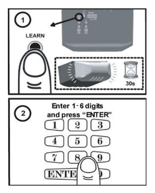
**STEP 1**: Locate the Learn Button (YELLOW) on the back of the Guardian Operator and press the button one time. You will hear 1 beep or the operator light will flash once to confirm the Guardian door operator is now READY to LEARN a new code. You will have 30 seconds to enter your code.
