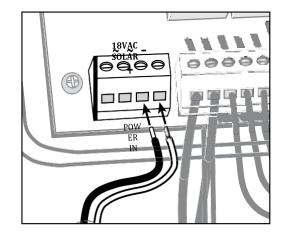
Insert one transformer wire into an 18VAC terminal. Insert the other transformer wire into the remaining **18VAC** terminal (see illustration). Transformer wires can be connected to the **18VAC** terminals regardless of color.
