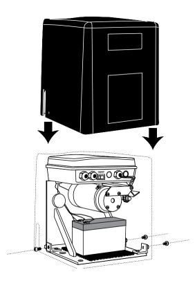
Mount the operator housing after all installation procedures are complete. Slide operator housing over legs, align holes, and use screws provided to attach housing to operator.
