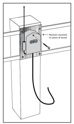
Check the range of the receiver before permanently mounting it. You may have to try different locations before permanently mounting the receiver. The receiver range can vary from 50 to 100 feet depending upon weather, topography, and external interference.
