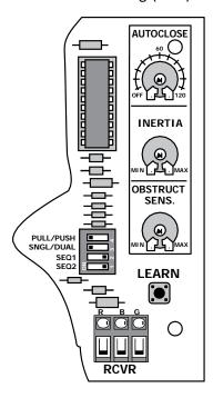
**AUTO CLOSE** (auto close timer): Determines how long the gate will remain open before it automatically closes. The limits are **OFF**, or from 3 to 120 seconds. The factory setting is **OFF**.
