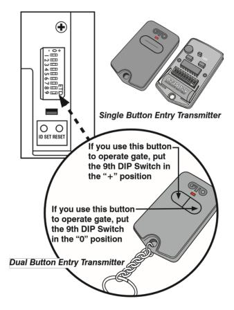
Change the Keypad's DIP Switch Settings NOT the Entry Transmitter Dip Switch Settings
