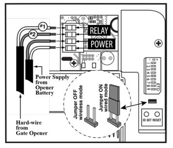
**Step 5:** Connect the jumper between the two terminals on the keypad control board (ON) as shown. **Step 6:** Slide the keypad into the cover and lock.
