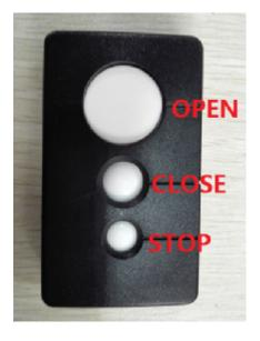
When the opener lights flash,release all button. Test by pressing the large (open) button on the remote, The door should open. Press it again while the door is open and nothing should happen. Press the middle (close) button and the door should close. Press the third (stop) button while the door is moving and it should stop immediately.
