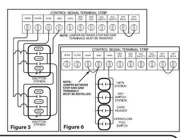
**AWARNING:** If momentary contact control is to be used, a monitored external reversing device such as a photocell system or sensing edge switch must be used. See pages 5.6-5.7 for installation of entrapment protection devices.
