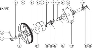
OUTPUT SHAFT ASSEMBLY (INDIRECT)
