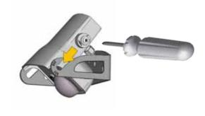
Position the sensor on the bracket and fasten the angle adjustment screws.
