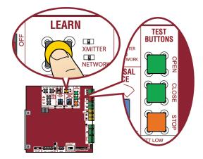
There are 3 different options for programming the remote control depending on how you would like the remote control to function. Choose a programming option:
