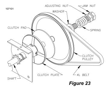
IMPROPER ADJUSTMENT OF CLUTCH SETTING COULD CAUSE ENTRAPMENT, INJURY OR DEATH. SET CLUTCH ADJUSTMENT FOR JUST ENOUGH FORCE TO OPERATE THE DOOR RELIABLY, BUT NO STRONGER. Contact a service professional to correct any binding, sticking or other door problems. DO NOT OVER-ADJUST CLUTCH SETTING TO COMPENSATE FOR A POORLY WORKING DOOR.
