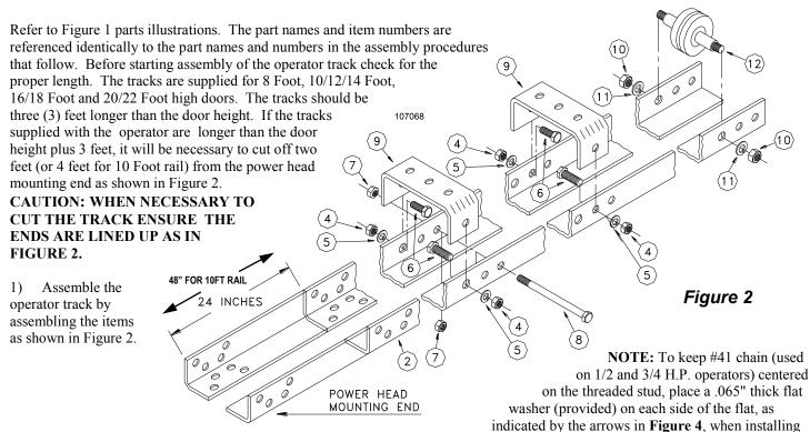
2) After the track is assembled, position track assembly onto the operator power head and attach with four 3/8"-16 x 1" bolts, lock washers and nuts (supplied in a separate hardware package #100470).
