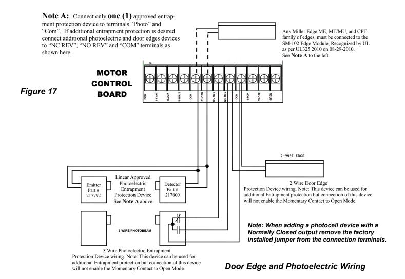
After properly connecting an approved Entrapment Protection Device (see above and Page 3) to the operator, see Page 15 for setting of the selector switches. These switches must be properly set and an approved photoelectric device or approved door edge device connected to the operator to obtain B2 Mode of Operation, Momentary Contact to Close.
