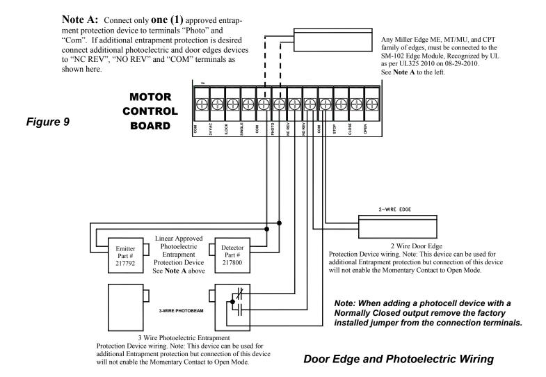
After properly connecting an approved Entrapment Protection Device (see above and Page 3) to the operator, see Pages 15 & 16 for setting of the selector switches. These switches must be properly set and an approved photoelectric device or approved door edge device connected to the operator to obtain B2 Mode of Operation, Momentary Contact to Close.
