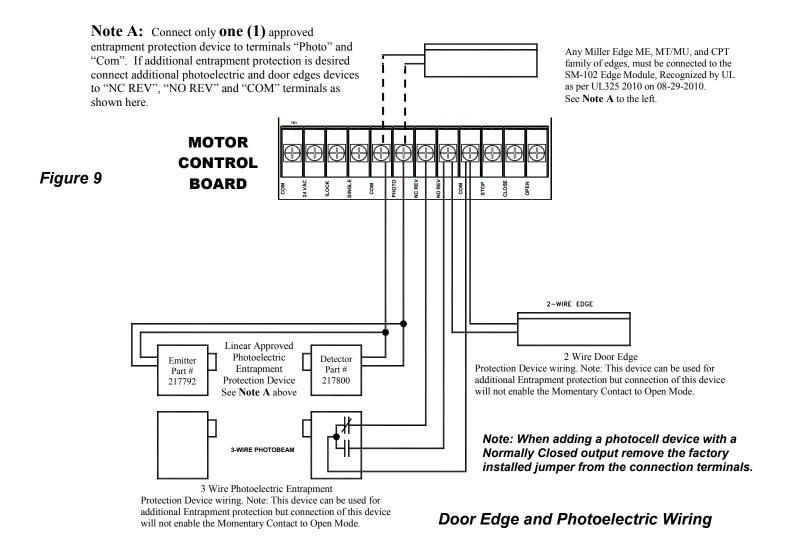
After properly connecting an approved Entrapment Protection Device (see above and Page 3) to the operator, see Page 16 for setting of the selector switches. These switches must be properly set and an approved photoelectric device or approved door edge device connected to the operator to obtain B2 Mode of Operation, Momentary Contact to Close.
