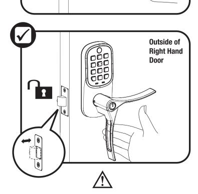
Test thumbturn and both levers in locked and unlocked positions. If operation fails, check installation beginning with Step 2 and refer to Hardware Troubleshooting.
