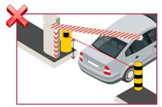
If the 0° reference beam is too low or too high, vehicle contact with the barrier may occur.
