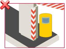
Do not cover the front face of the sensor with glass or plastic.
