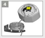
Firmly close the protection cover. Do not pinch the cable.
