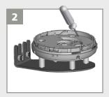
Position the bracket and secure using the 4 screws to avoid vibrations.
