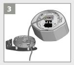
Open the protection cover, plug the connector and position the cable in the raceway.
