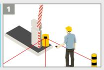
Activate the visible laser beams by remote control to position the sensor fields correctly.
