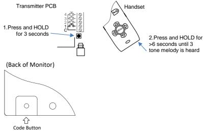
Once the melody is heard, the handset / monitor should then be working. The system should now be ready for testing.
