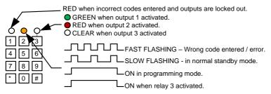
**TIP**: After power up, as a security precaution, the keypad cannot be programmed for 60 seconds. Once this time elapses, you may begin.
