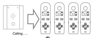
Answer the call on any handset by pressing (), and check for good 2 way speech. Adjust volume while on a call with up and down arrow buttons on the handset and press the same button again to end the call. The gate/door release button can be pressed at any time, either while on or off a call. The relay on the transmitter should then pulse on for 4 seconds.
