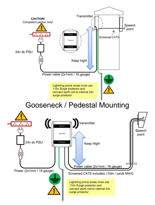
**Tip:** For shorter distances, some installs may mount transmitter on pedestal for convenience. Range test first! For high security applications, it is recommended to locate the transmitter INSIDE the property perimeter.
