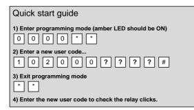
**Tip:** The engineer code must be the same length as user codes. So if using a 6 digit engineers code, then user codes must also be 6 digits long etc.
