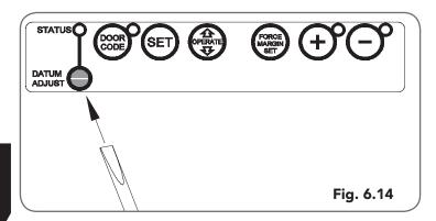
NOTE: If the status LED is already illuminated when power is connected then turn the datum adjust screw until the LED goes off then turn back one notch to illuminate again.
