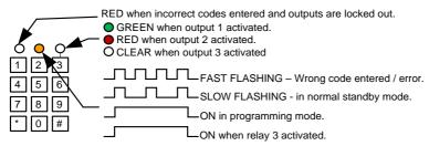
**TIP**: Amber light flashes to indicate standby mode. **TIP**: Simply enter your code to trigger gates or door.
