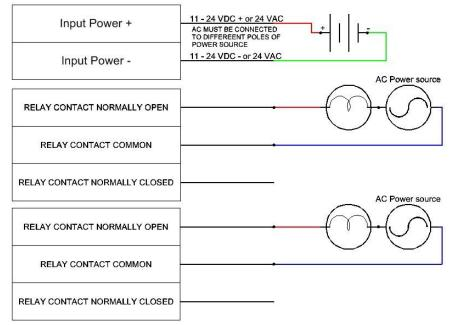
2. To open a gate or door using channel 1 and close with channel 2.
