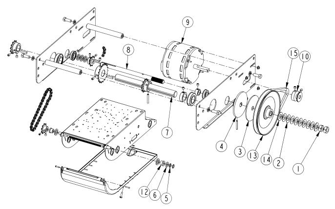
Figure 33 - OMT Mechanical Exploded View
