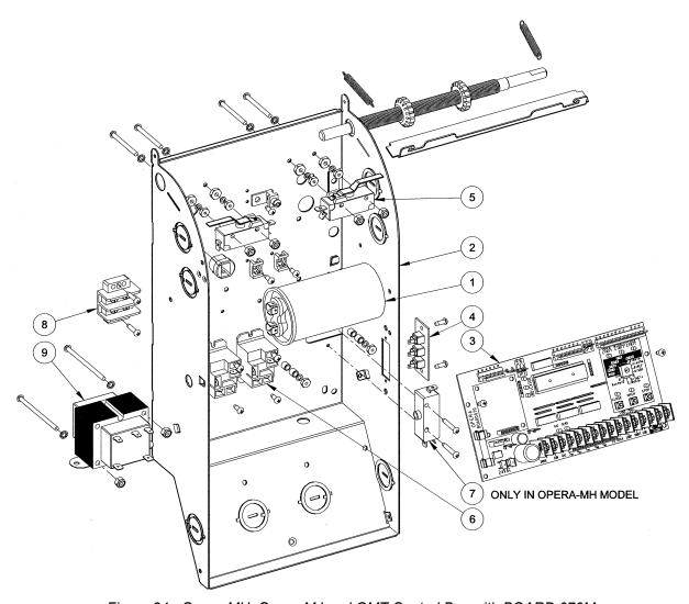
Figure 34 - Opera-MH, Opera-MJ and OMT Control Box with BOARD 070M
