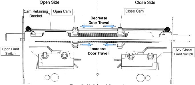
Figure 5 - Limit Cam Adjustment
