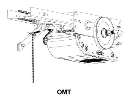
Commercial & Industrial Medium Duty Trolley Operator (For standard lift sectional doors)
