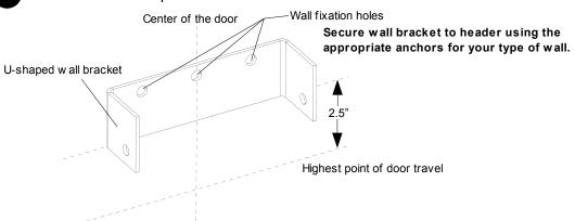
4 Attach tracks to U-shaped wall bracket
