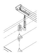
Door arm should ideally hang vertically when the door is closed.
