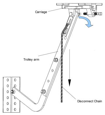
Figure 4 - Disconnect Trolley Arm From Carriage
