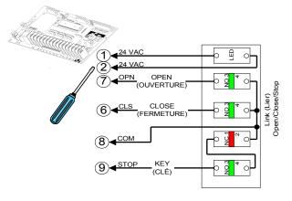
Figure 10 - STATION 080 3-PBS Open / Close / Stop with Key Lock-out and Light
