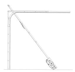
Allow the motor to rest on the floor and raise the front end of the rails and secure with the bolts and nuts (do not tighten).
