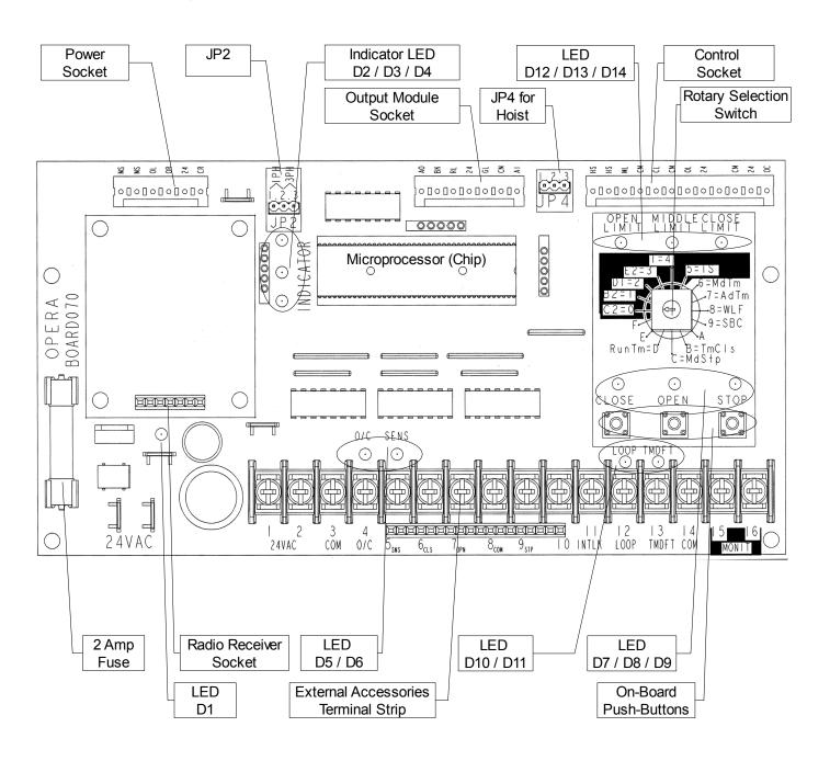
Figure 30 - Electronic Control Board - BOARD 070M
