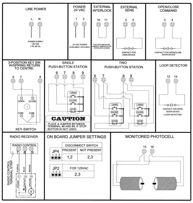
Figure 32 - External Wiring
