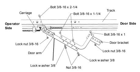
Attach door arm to door using appropriate fasteners. Mount door bracket to the center of the door.
