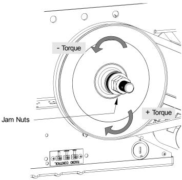
Figure 29 - Clutch Adjustment
