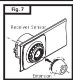
Note: Sensor alignment must be done with the door in the closed position in order to ensure proper visibility of the sensor indicator LED. Accurate alignment will ensure a high standard of safety and performance.
