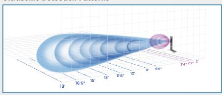
Microwave detection patterns (blue above) are adjustable from 7 to 18 feet. The Ultrasonic Sensor is for close range detection (purple). The OVS-01GT Vehicle Virtual Loop also features 5 sensitivity settings.
