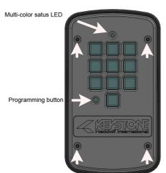
4 screws for batteries replacement
