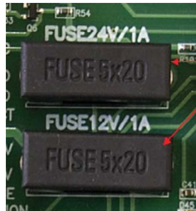
CIRCUIT BOARD POWER INDICA- TOR LED LIGHT AND PROTECTION FUSE
