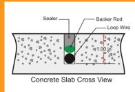
Cut 1" deep cut in existing surface, place 45° cut at the corners to relieve stress on the wire. Notch out for the "T" and place into the saw cut. Place backer material into saw cut over loop wire and push down tightly. Place a good grade sealer over the saw cut to
