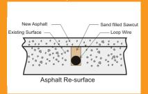
Saw cut existing surface 3/4" deep and place loop into bottom of saw cut. Place sand over loop wire to surface of existing surface and pack tightly. Lay new asphalt.
