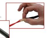
Position the 8" piece of Shrink Tubing centered over the 4" piece of Shrink Tubing and glue tapes. Then shrink the 8" piece of Shrink Tubing using a Heat Gun or Blowtorch\*.
