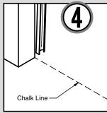
4. Snap a chalk line from jamb to jamb at the location that the door meets the opening when closed.
