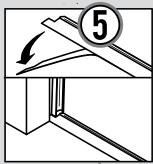
5. Install Storm Shield®along chalk line removing liner and patting the seal down 6-8" at a time. ONCE STORM SHIELD® COMES IN CONTACT WITH THE CONCRETE IT CANNOT BE RE-POSITIONED.
