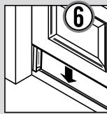
6. Garage door should be lowered on Storm Shield<sup>®</sup> and allow 24 hours for adhesive to take a set. Use a small roller to aid the adhesive in making contact with the floor if possible.
