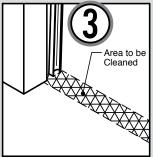
3. Use a lint free cloth to clean floor with Acetone, as it will aid in removing moisture from the surface of the concrete. If Acetone is not availale, Pine-Sol® can be used. Note: If using Pine-Sol® floor must be completely dry before applying Storm Shield<sup>®</sup>.
