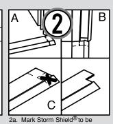
notched by aligning end with outside of vertical track and marking in line with inside of track. 2b. Align Storm Shield® with jamb against vertical track. Mark backside of vertical track as shown 2c. Cut X portion to notch
