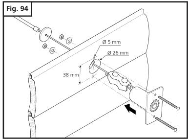
Locate mounting position for emergency release system lock. Mark and drill 5mm and 20mm holes per Fig. 94. Install and secure lock with hardware provided.
