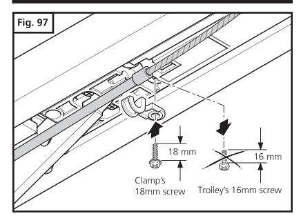
Install cable securement clamp (Fig. 97). Make sure to replace trolley's 16mm screw with 18mm screw provided with clamp.
