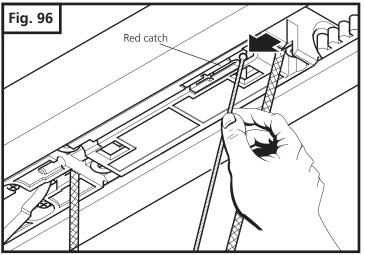
Insert cable in the trolley's red catch as shown on Fig. 96.
