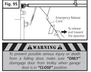
Unlock trolley by pulling Emergency release cord toward the operator as shown on Fig. 95.
