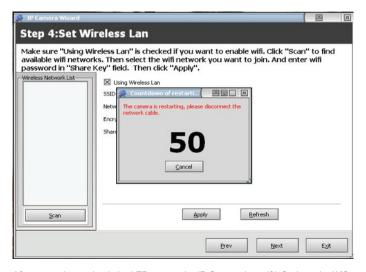
After count down, check the LED next to the IP Camera lens. If it flashes, the Wifi connection successful, you may click "Exit". It is stays off, the wifi fail please verify the SSID / Password info
