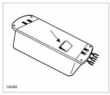
The Receiver Coding RECEIVER: Switches can be accessed by removing the small door from the back of the Receiver using a small screwdriver or
