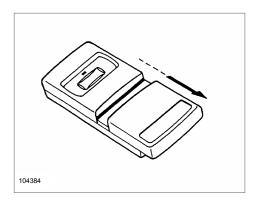
**TRANSMITTER:** To gain access to the Transmitter Coding Switches, remove the Battery Cover from the front of the Transmitter by sliding it toward the bottom of the Transmitter as illustrated.
