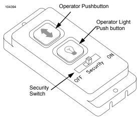
1. Operator Pushbutton — Red-backlighting. Used to start or stop the operator. The function of this pushbutton is automatically disabled when the Security slide switch is set to the "ON" position and the door is fully closed.
