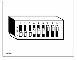
**CODING BLOCK:** Transmitter Receiver Coding Switches are contained in identical Coding Blocks, consisting of nine small switches, labeled 1 - 9, each of which can be set in any of three positions, labeled +, 0, -
