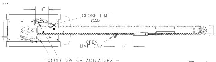
**STEP 11:** On most models, the Limit Cams are installed at the factory. If the Limit Cams have not been installed, fasten them to the Chain in the approximate positions illustrated above. Position the Switch Actuators as shown above.
