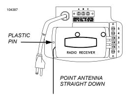
Mounting The Receiver: After setting the Coding Switches, mount the Receiver on the rear panel of the Opener by connecting it to Terminals 1, 2 and 3. A small Plastic Pin is provided to secure the other end of Receiver to the panel. For proper operation, the Antenna Wire should be POINTED STRAIGHT DOWN toward the floor.
