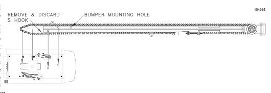
**STEP 7:** Install the Rubber Bumper into its mounting hole on the Tee Rail (see illustration above for location). Secure the Bumper to the bottom of the Tee Rail using one 5/16"-18 X 1" hex head bolt and one 5/16"-18 washered nut (supplied) Tighten the bolt a MAXIMUM of 1.5 turns after the bolt and nut are snug.
