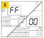
Display will toggle between FF and DD for 5 seconds.
