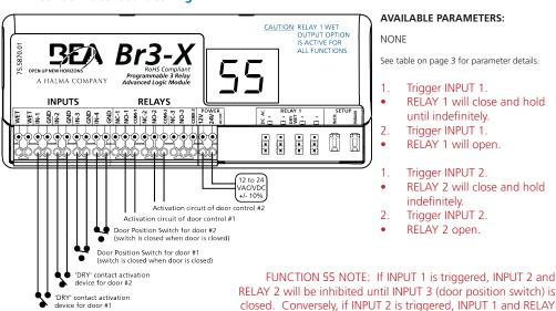
1 will be inhibited until INPUT 4 (door position switch) is closed.
