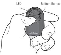
4 On the remote control, press and release the button that you would like to program twice. The blue LED will blink for up to 60 seconds.
