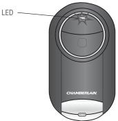
Test the remote control by pressing the button you programmed in step 4. If the garage door opener, commercial door operator, or gate operator does not activate, repeat the programming steps.
