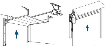
2 Press and hold bottom button on the remote control until the blue LED stays solid (approximately 15 seconds) then release the button.
