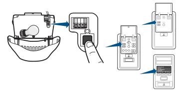
When the garage door begins to open, immediately press 5 and release either of the buttons on the remote control to confirm the code and exit programming.
