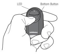
**4** On the remote control, press and release the button that you would like to program twice. The blue LED will blink for up to 60 seconds.
