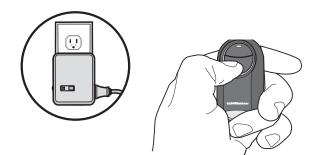
On the remote control, press and release the button that you would like to program twice. The blue LED will blink for up to 60 seconds.
